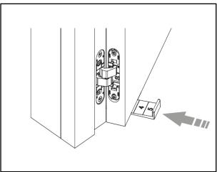
2. Using a wedge (an adjustment washer for doors), lift the door to the desired height in such a way that the gap between the door frame and the leaf is about **3 mm**. Then tighten all hinges to the leaf.
