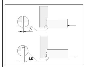
The range of hinge adjustment in this plane is +/-1.5 mm
