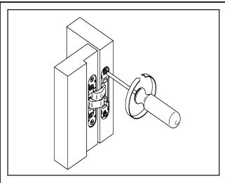
In order to adjust the leaf height (decrease or increase the top gap), loosen screws in openings [A] that hold all hinges in the leaf
