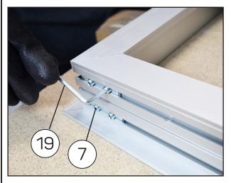
C. Tighten the angle brackets [7] using the hex key [19], ob serving the correct alignment of profiles with each other
