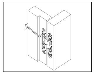
3. In order to adjust the leaf so that its surface is flush with the wall surface, first loosen [D] bolts
