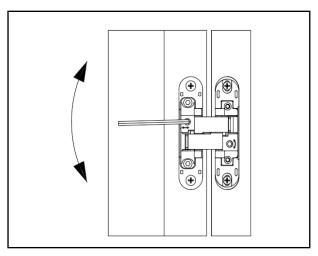
4. Then move the leaf closer to or farther from the door frame by rotating [C] bolt. After adjusting the hinges in this plane appropriately, again tighten [D] bolts to lock the position
