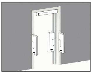
H. After mount frame in the wall again check vertical and horizontal placement (and dismantle the expansion strips [7] if they were mounted)
