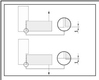
The range of hinge adjustment in this plane is +/-1 mm
