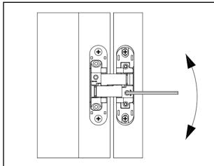
5. In order to adjust the gaps between the leaf and the door frame on the sides, tighten or loosen [B] bolt in the hinge, which makes the leaf move right or left.
